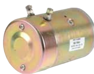
10739N Motor - Pump 12 Volt, CW, 9-Spline Shaft, Insulated Grd.
